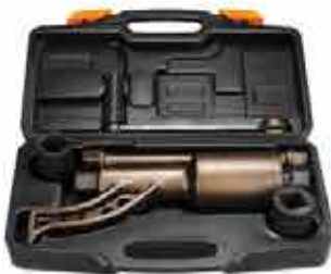
MH-68C-C Trans-speed ratio: 1:68 Max torque output: >6200N.M Drive square: 1" Weight: 8.5kg Material: 40Cr Sockets: 1-4pcs
